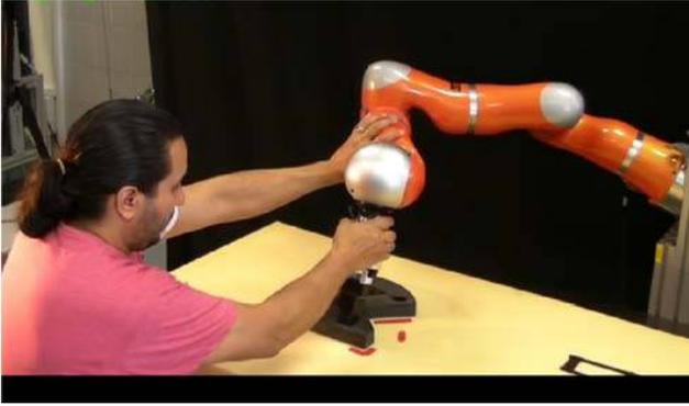
torques and transform them into the corresponding tool center point forces and torques. We take care that the workspace configuration does not change during this process and since our robot can accurately track the joint space trajectories, the measured forces and torques provide a good reference for later adaptation.
