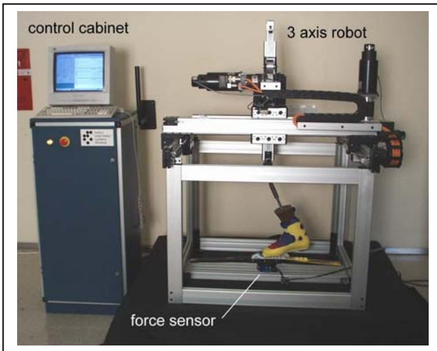
**Figure 3** Robot for testing ski boots
