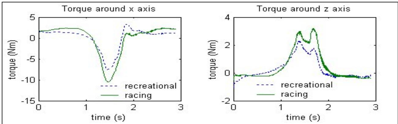
**Figure 7** Comparison between torques measured on recreational and racing ski boot during the simulation with the robot
