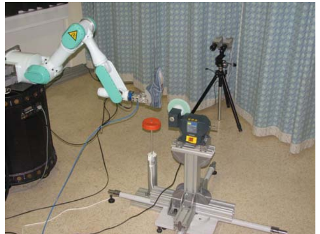
Fig. 5. experimental cell for shoe bottom roughing
